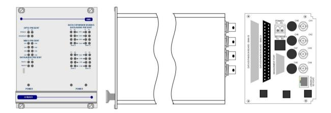
The **AMG4748AR-SF** is a rackmount four channel video receive unit designed to receive 4 video signals and transmit and receive up to 8 data or audio signals over one singlemode fibre. The 8 data/audio channel interfaces, whether RS232, RS422, RS485, 20mA, TTL, Contact Closure, Lonworks or Audio, are defined at manufacture by the addition of daughter boards fitted onto the Data Expansion Board A.
